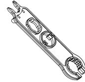
Extractor de conector fotovoltaico\*1
